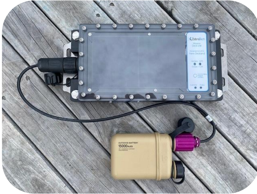
External power version Deck Unit charging from power bank
