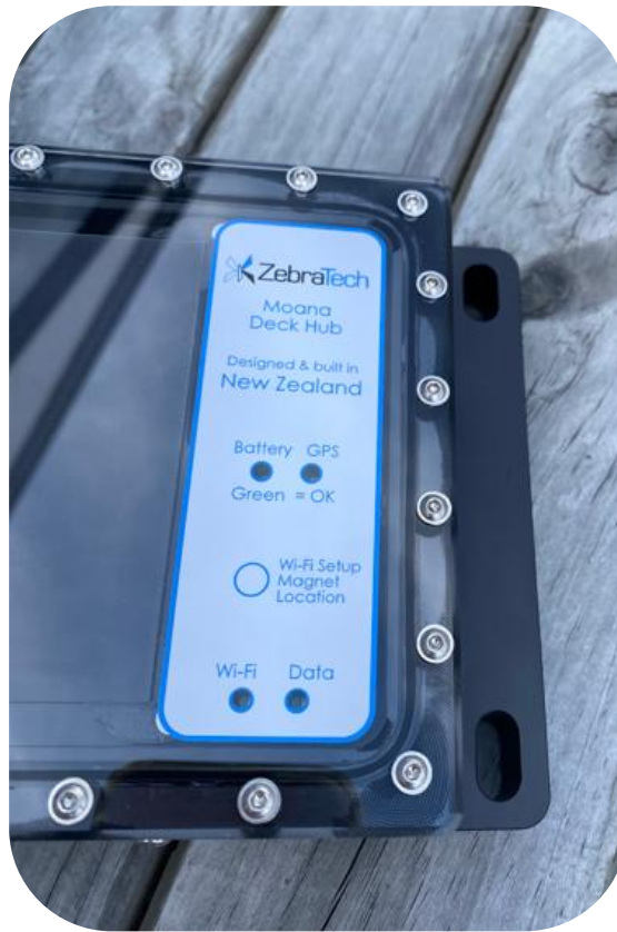
Deck Unit status indicator panel
