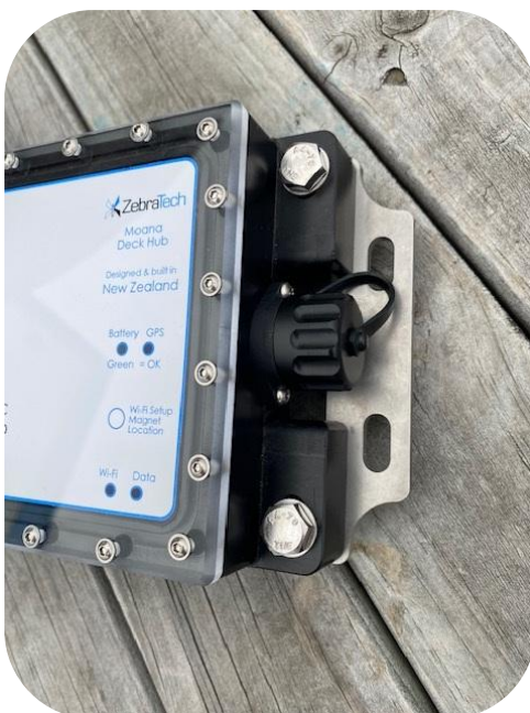
Moon pool Deck Unit external power connector with protective cap fitted
