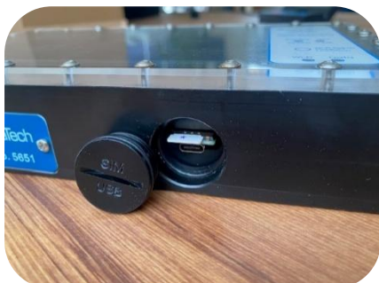
Round port SIM slot and USB charging port (Serial number 5546 onwards)
