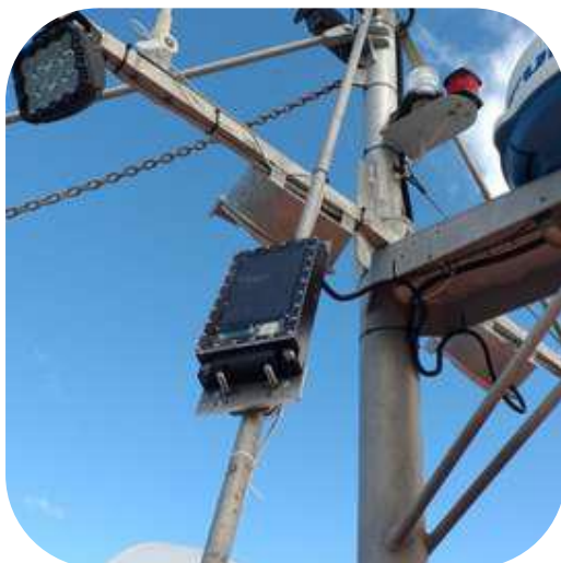
Deck Unit mounted at 45 Degrees to minimise heating in hot climates
