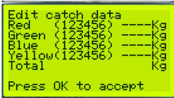
Enter the catch from that dive event for each diver and then push the OK button. The cursor will drop down to the next diver so enter their catch. If necessary you can use the RED button to arrow back up to redo a diver's catch figures.
