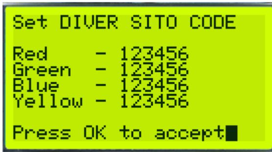
To allocate a diver to the colour RED, push the RED button and then move the cursor to the left hand side of the numbers by pushing the LEFT arrow (the yellow button). You can now type a diver's 6-digit SITO ID on the keypad. Push OK to accept. Enter the next diver's SITO ID, etc.
