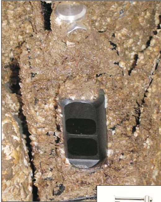
Hydro-Wiper protecting a Seapoint Turbidity Sensor from heavy biofouling
